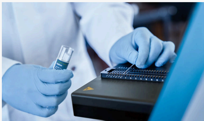
Figure 4. Easy sample introduction with capillaries.
