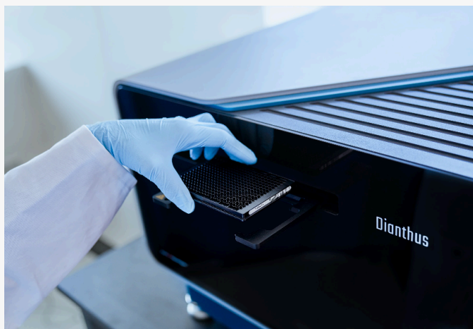
Figure 3. Manual loading of 384-well microplate.
